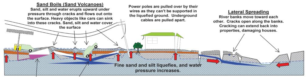
Tanks, pipes and manholes float up in the liquefied ground and break through the surface. Pipes break, water and sewage leaks into the ground.
